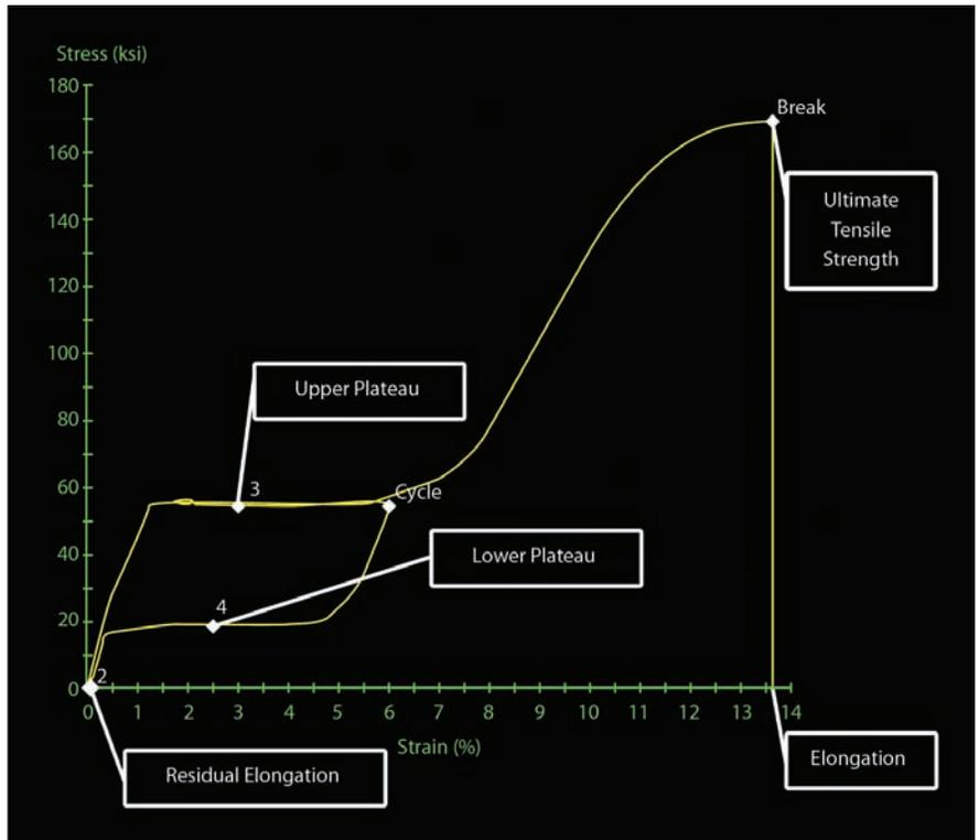
Fig. 3 – Typical Nitinol Tensile Test. In addition to the ultimate tensile strength and elongation that are common to other materials, there are other critical parameters that are measured when testing Nitinol. Upper plateau strength, lower plateau strength and the residual elongation (or permanent set) are also recorded.
