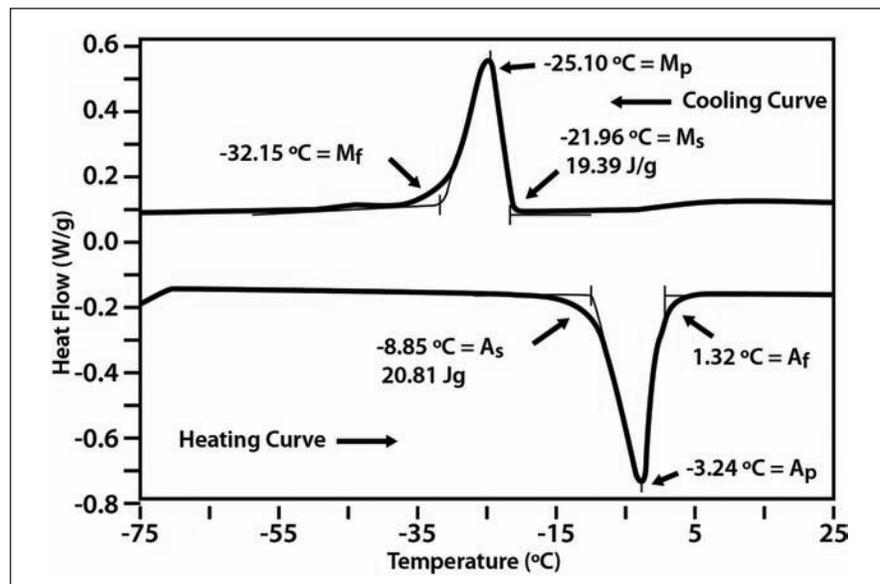
Fig. 2 - Various transformation temperature measurements of the Nitinol ingot are recorded by a Differential Scanning Calorimeter (DSC).
