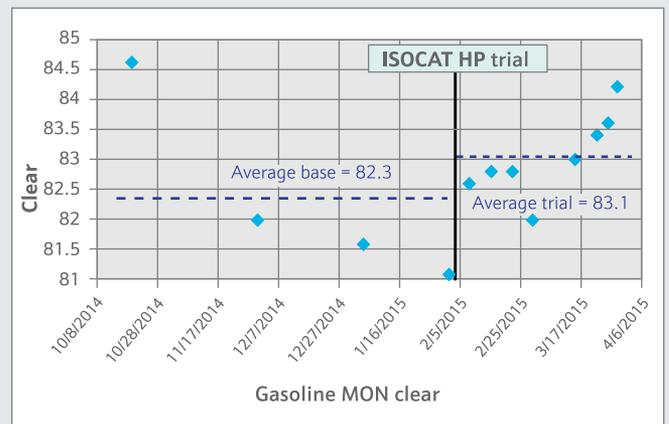
**Figure 3.** Time plots show octane response during ISOCAT HP trial.
