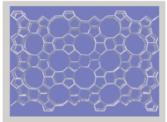
**Figure 2.** The shape-selectivity of ZSM-5 crystal pores and channels.
