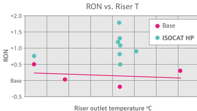
**Figure 4.** Cross-plots showing RON octane increase at fixed single variables during the ISOCAT HP trial, riser outlet temperature (°C).
