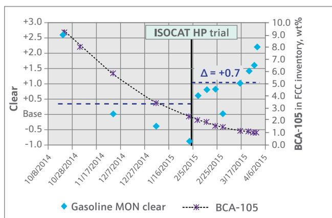
**Figure 6.** Impact on gasoline octane following conclusion of BCA-105 trial.
