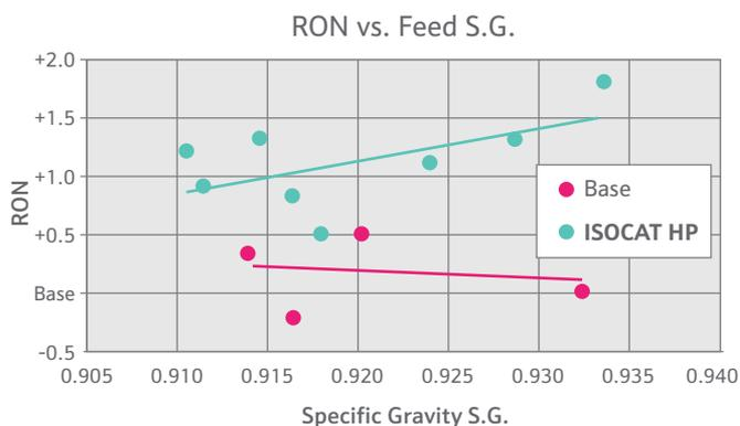
**Figure 5.** Cross-plots showing RON octane increase at fixed single variables during the ISOCAT HP trial, specific gravity.
