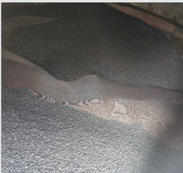
Disturbed two-layer catalyst bed
