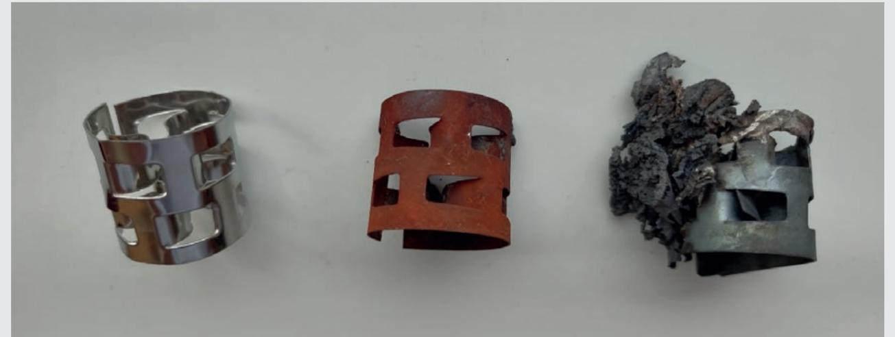
Figure 3: Pall rings – new (left), with iron oxide deposits (middle), and after a fire (right)
