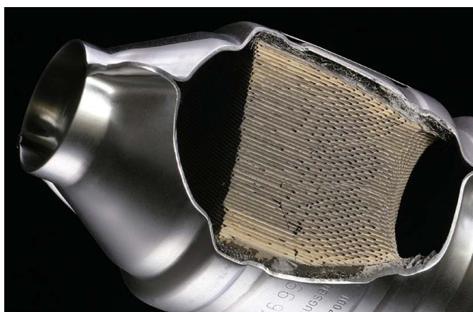
Figure 8 Automotive emissions control catalyst cutaway, showing the can containing the PGM-coated support
