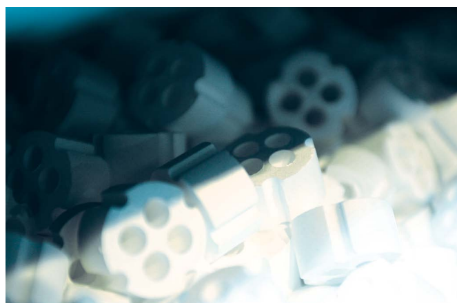
Figure 9 An example of a PGM process catalyst, comprising pellets of support material carrying very small quantities of PGM catalyst
