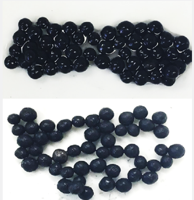
Figure 8: Photos of mercury-laden PURASPEC after exposure to water (left) and after subsequent tumbling in a Pascal mixer (right).
