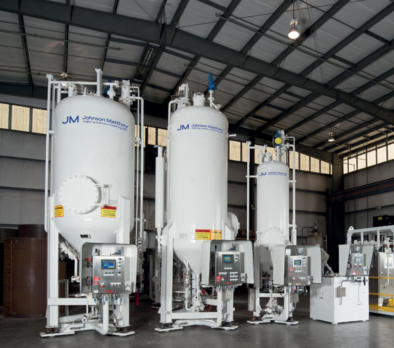
When refilling, carrier air is usually vented to atmosphere. To prevent any fines escaping, the **INTERCAT** loader is fitted with a sintered metal filter (SMF). This is a stainless steel mesh self-cleaning system which prevents any powder escaping the addition system during refill. There is a back pulse system that cleans the filter while in operation and blows back the fines into the vessel.
