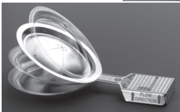
Rupture disc. Different layers from bottom-up: Vacuum support, Seal, Slot cover, Top section and Protective ring (optional).
