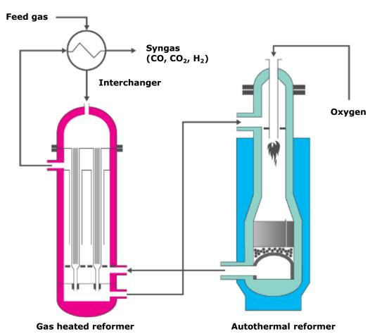
**Methane** (CH<sub>4</sub>) from natural gas is reacted with steam to produce **hydrogen** (H<sub>2</sub>) and **carbon dioxide** (CO<sub>2</sub>)
