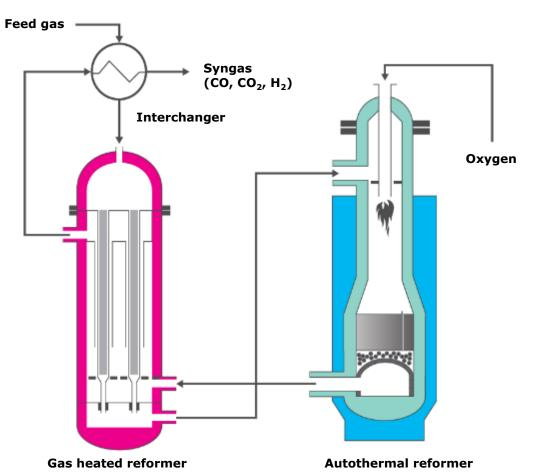
**Methane** (CH<sub>4</sub>) from natural gas is reacted with steam to produce **hydrogen** (H<sub>2</sub>) and **carbon dioxide** (CO<sub>2</sub>)
