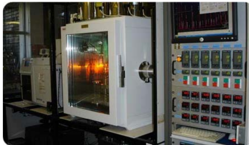
Micro reactors used to simulate large scale FT operating conditions
