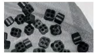
→ Platinum gauze catalyst for nitric acid manufacture and catalyst pellets for the abatement of nitrous oxide from nitric acid plants.
