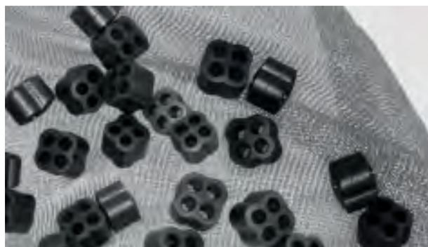
→ Platinum gauze catalyst for nitric acid manufacture and catalyst pellets for the abatement of nitrous oxide from nitric acid plants.
