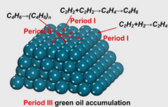
Molecular modelling of palladium crystallites, determining the oligomerisation pathway for the formation of green oils.
