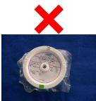
The reels should be stored in the 'rolling position' to ensure that the layers of wire do not tangle.
