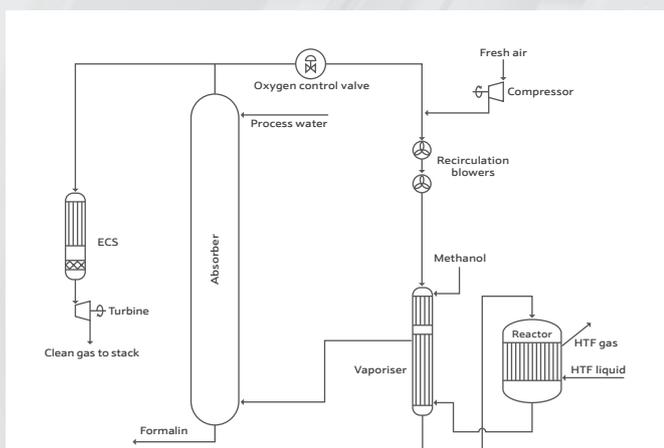
**Figure 1:** Location of the oxygen control valve in a turbocharged plant
