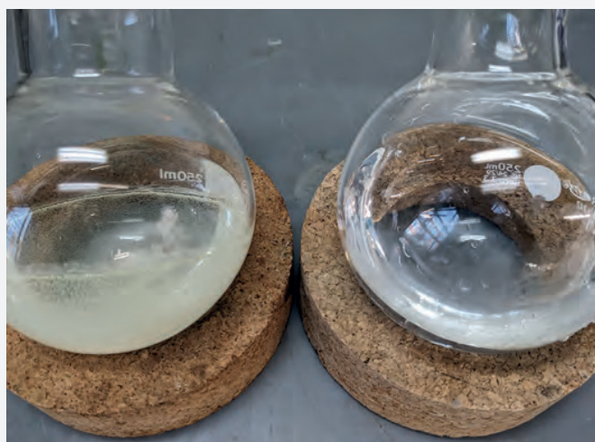
Figure 2. Soxhlet extraction in hexane solution. PURASPEC 2058 (right) and iron oxide (left).
