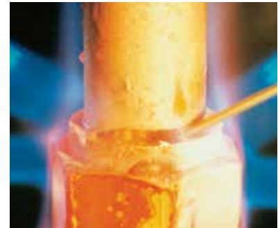
Flux protects the component from oxidation as the brazing filler metal flows
