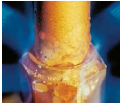
The flux becomes clear and watery as it approaches brazing temperature
