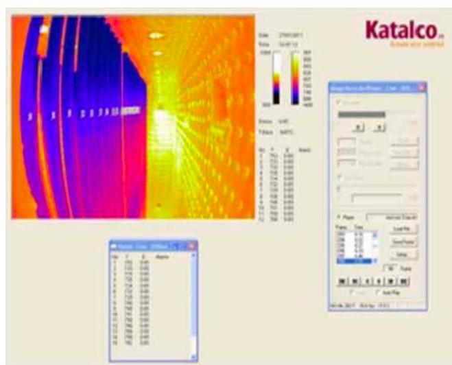
Figure 1. Snapshot of video from Reformer Imager
