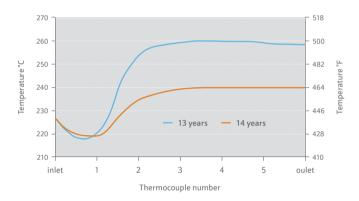
The temperature profile after 13 and 14 years continuous operation showed no movement of the profile in the year, and the required < 10 ppm carbon oxides slip has been maintained throughout and the inlet temperature is still only 220°C (428°F).
