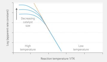
Under these conditions, film diffusion controls the overall rate of reaction. Diffusion limitations can be overcome to some extent by the use of a smaller particle size, such as **KATALCO** 11-4M, to provide a higher geometric surface area to enhance mass transfer.
