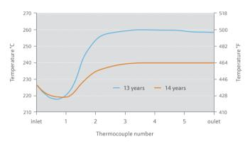
The temperature profile after 13 and 14 years continuous operation showed no movement of the profile in the year, and the required < 10 ppm carbon oxides slip has been maintained throughout and the inlet temperature is still only 220°C (428°F).
