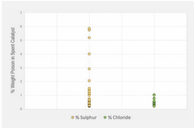
Figure 10: Levels of sulphur and chloride measured in spent LTS catalysts
