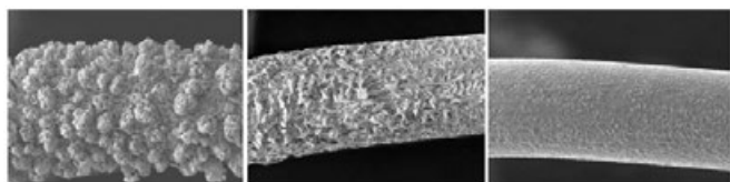
Figure 2. Layers 1, 3 and 5 of a catalyst pack composed of 5% rhodium 95% platinum alloy after 5 days operation at 4 bar g showing a high level of restructuring and cauliflower growth in the top layer and negligible restructuring on the bottom layer. Images are at 4000 times magnification (23).
