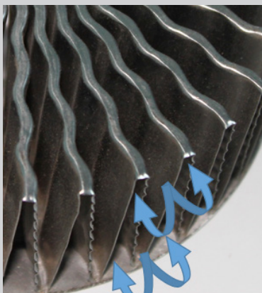
Figure 3. Gas forced out of duct and back into the underside vents
