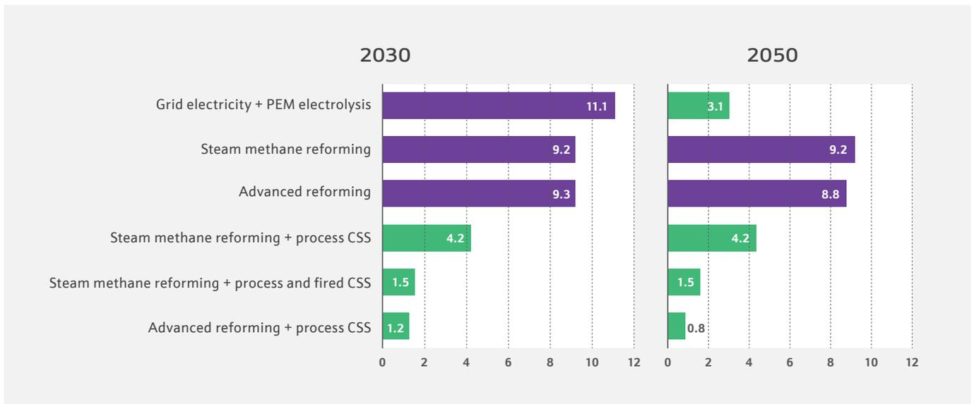
Figure 4. Greenhouse gas emissions from different hydrogen production pathways in 2030 and 2050 (kg CO<sub>2</sub>/kg H<sub>2</sub>)<sup>5</sup>.
