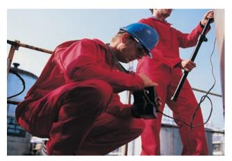
This measurement uses a radioactive neutron source and a neutron detector to measure neutron back-scattering and to detect density differentials in the material inside the vessel. As zinc sulphide is more dense than zinc oxide, there is greater neutron absorption through zinc sulphide than zinc oxide. This difference is measured and therefore accurately determines the position of the interface.
