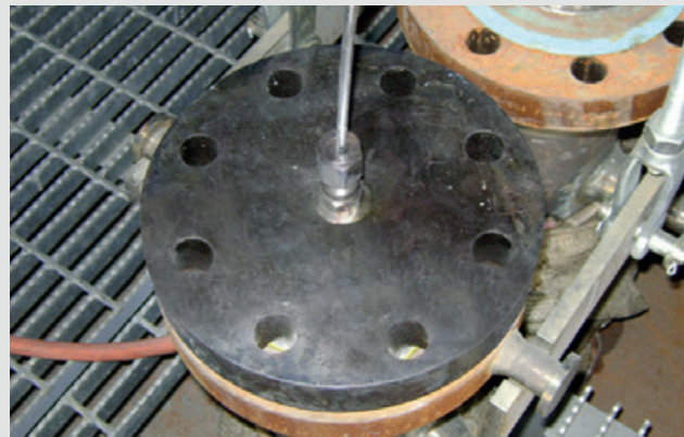
CatTracker installed in a reformer tube
