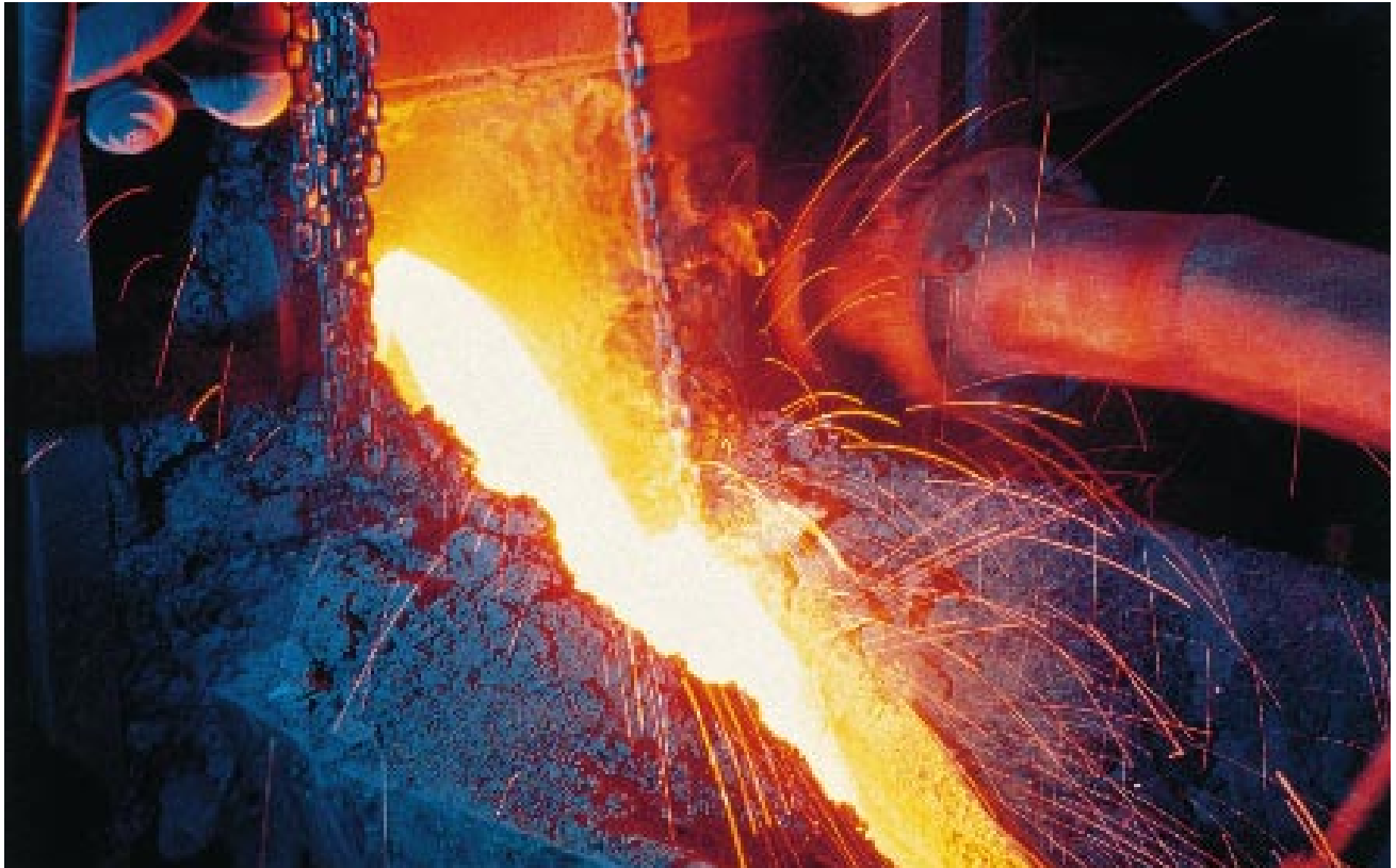
Molten matte containing palladium and platinum being poured at the Stillwater smelter
