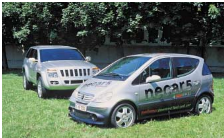
PEM fuel cells power advanced prototype vehicles such as DaimlerChrysler's NECAR 5 and Jeep Commander 2
