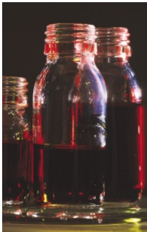
Samples of rhodium nitrate, a key component of many gasoline autocatalysts.
