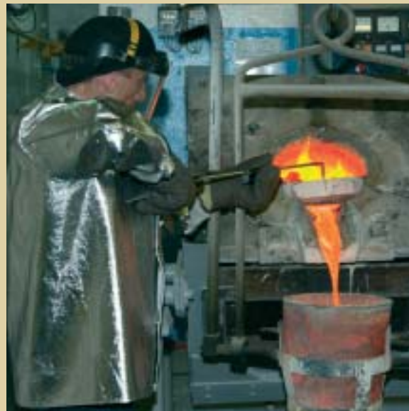
Tapping molten palladium at the Krastvetmet pgm refinery in Krasnoyarsk
