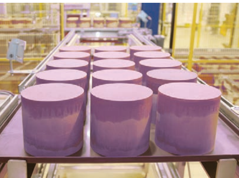
Catalysts for controlling pollution from diesel vehicle exhaust.
