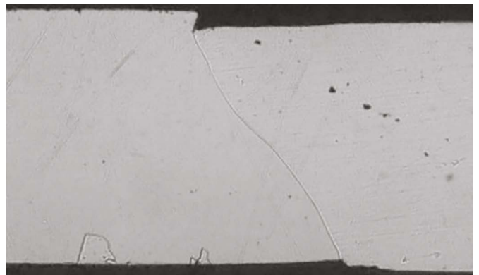
Standard Pt wire with grain boundary movement
