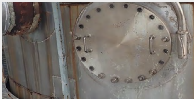
Figure 2: Water could be seen pouring out from the reactor through the temporarily closed manhole above the tube sheet
