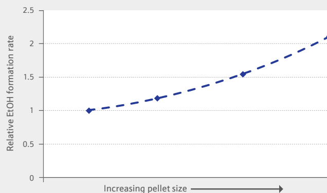
Figure 3: KATALCO 51-91 optimised for higher methanol selectivity and lower by-products
