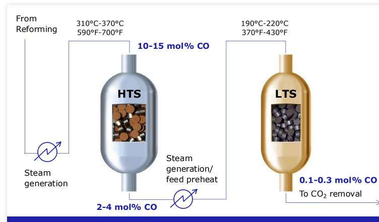
Reduce CO levels and increase  $H_2$  make CO +  $H_2O \leftrightarrow CO_2 + H_2$  (exothermic)
