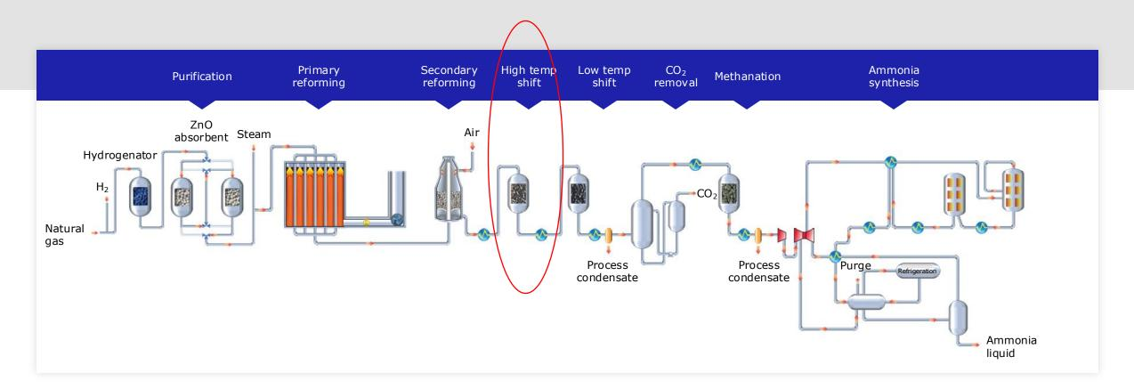
The WGS produces approximately 10-20% of the hydrogen
